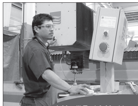
A Merrill Tool & Machine technician precision cuts a part with a WaterJet Cutting Table.
